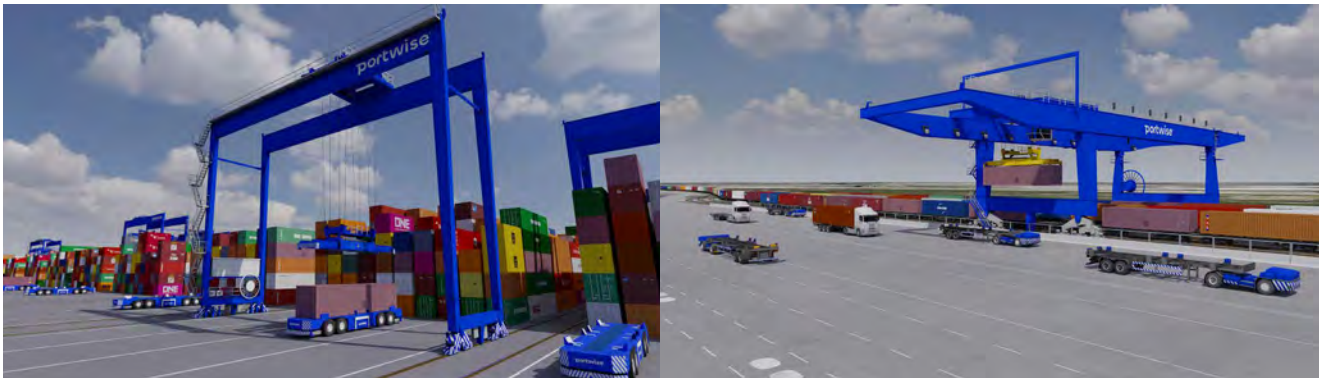
FIGURE 1: Cases with autonomous intelligent guided vehicles (IGVs) in a non-mixed traffic operation environment with perpendicular ASC yard (left) and autonomous terminal trucks in an intermodal site (right)
