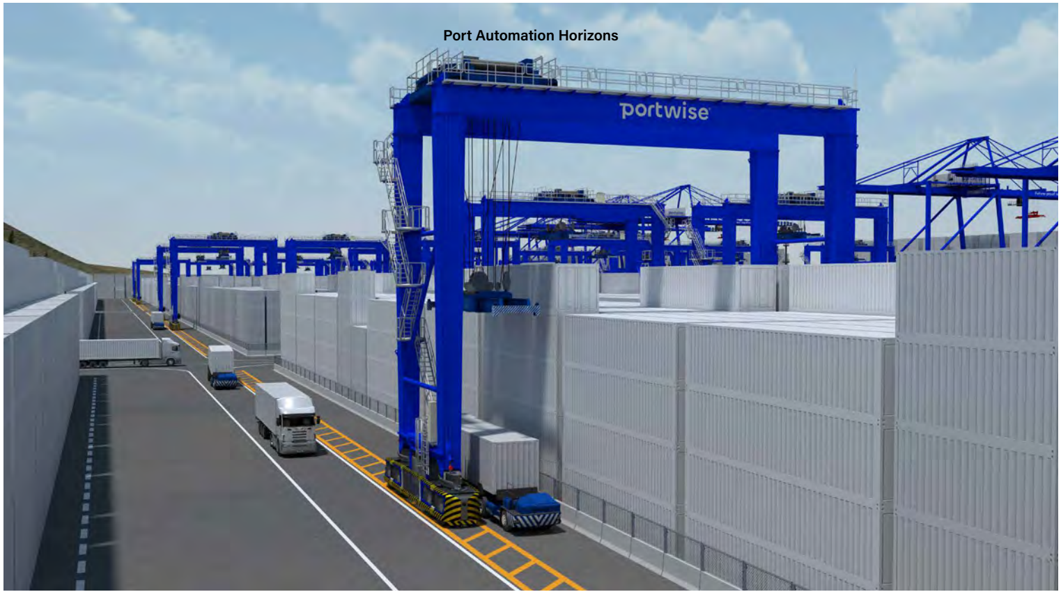
FIGURE 2: Modelling of autonomous terminal trucks mixing with road trucks in RTG yard (example of a 3D visualisation)
