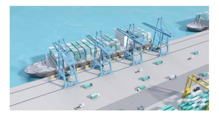
range or may be blocked by other obstacles, it is not always aware of the situation at the first several bays of the block. In case of a manual vehicle stopping at the first bay, AT may end up queuing behind and blocking the intersection. With V2X detecting the obstacle in advance, AT can choose the bypass lane or wait outside the intersection.
