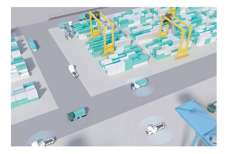
AT reports its state and local path in a constant frequency. FMS continuously checks the paths with conflict or deadlock. By setting the speed or reserving the lane segment, FMS can resolve any deadlock in advance and reduce any potential risks.
