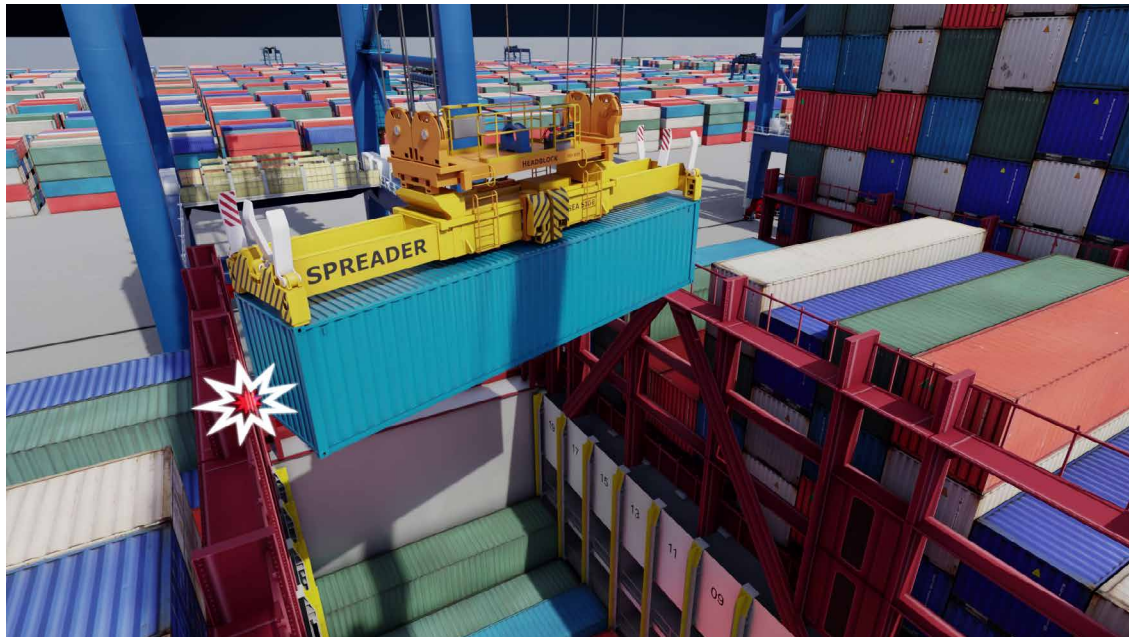
FIGURE 3. SIBRE Guardian. Impact detection by IMU technology
