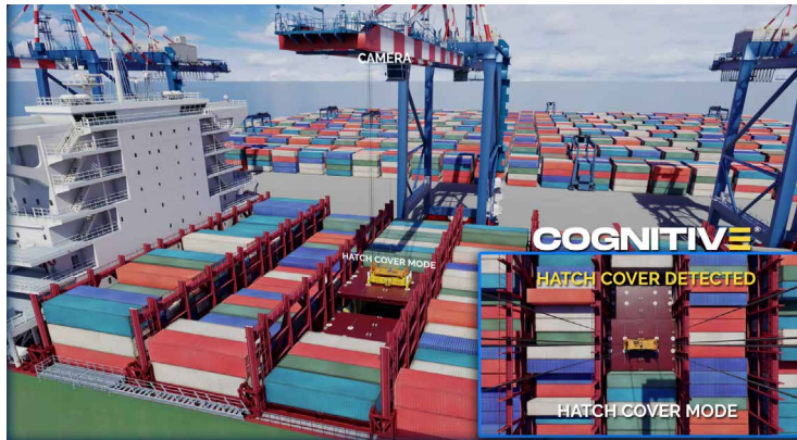
FIGURE 5. SIBRE Cognitive. Hatch cover detection by AI
