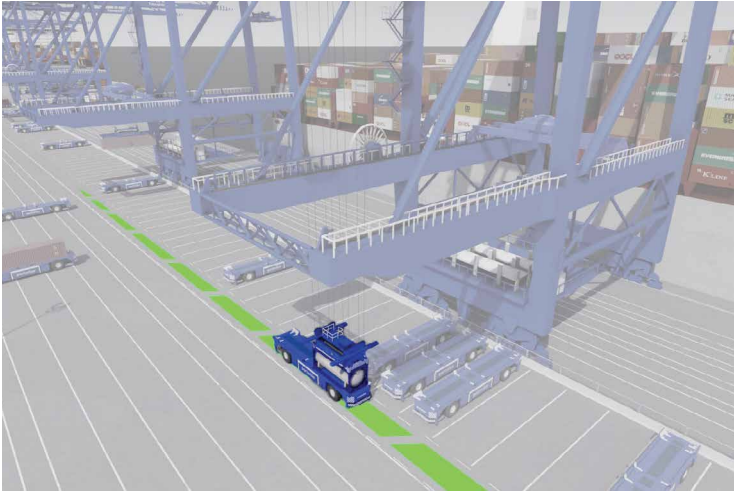
FIGURE 6. Exception lane for containers that cannot be handled with the second trolley
