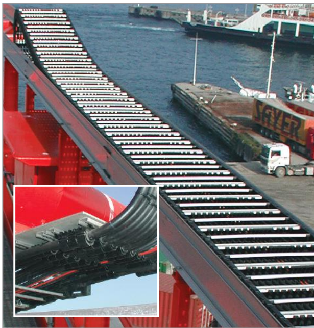
■ MC-crane cable with cable package, SZL strain relief driven-end plate and sea-watertight AL-guide channel for worldwide use in port cranes
