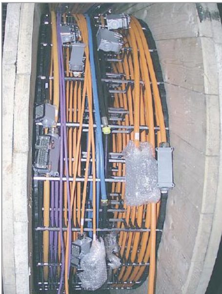
■ 125 m travel length: carrier fully harnessed with Series 700
