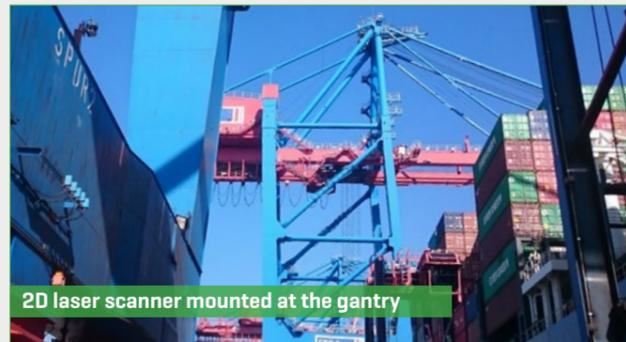
2D laser scanner mounted at the gantry
