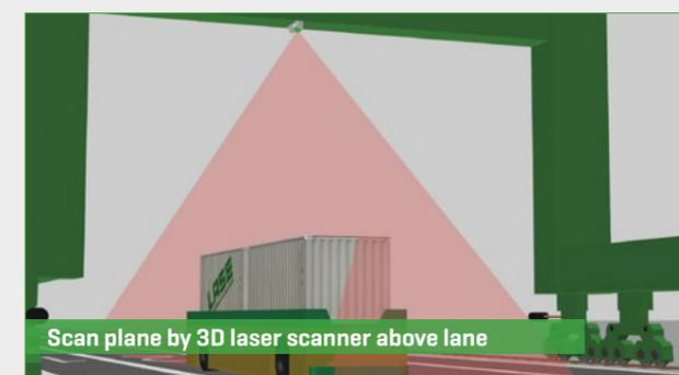
Scan plane by 3D laser scanner above lane
