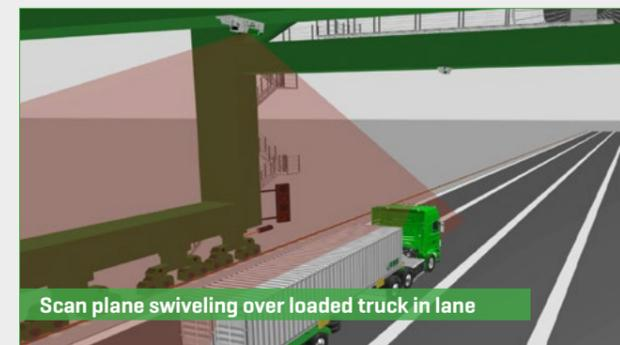
Scan plane swiveling over loaded truck in lane
