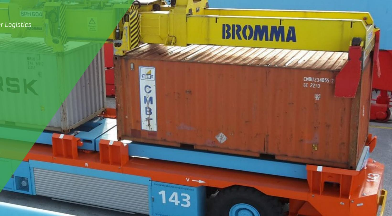
The measurement system LaseAVP -Automatic Positioning Vehicle is designed for STS-Crane operations for an efficient workflow in container handling while loading and unloading operations of vessels. The application is able to position AGVs for all common container types, e.g. 20ft, 40ft and 45ft and can also be utilised for twin-mode spreader operations under STS-Cranes.
