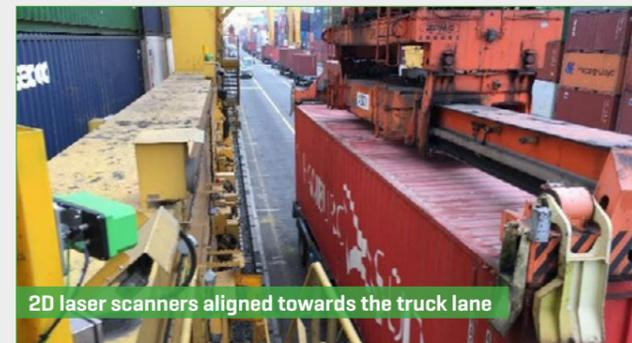
2D laser scanners aligned towards the truck lane
