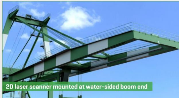
2D laser scanner mounted at water-sided boom end
