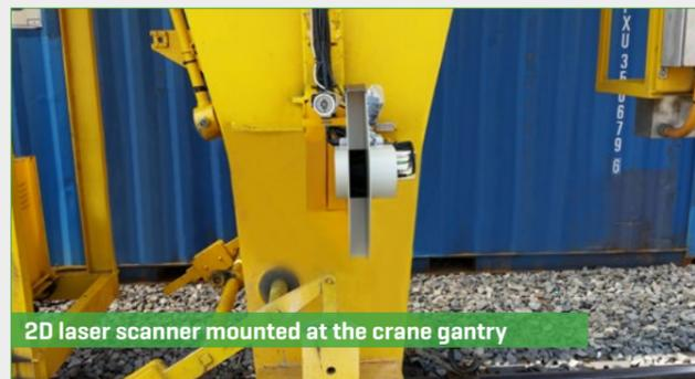
2D laser scanner mounted at the crane gantry
