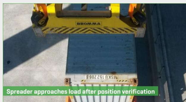
Spreader approaches load after position verification
