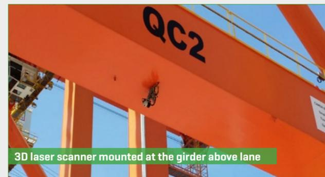
3D laser scanner mounted at the girder above lane
