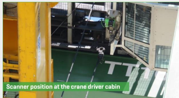
Scanner position at the crane driver cabin
