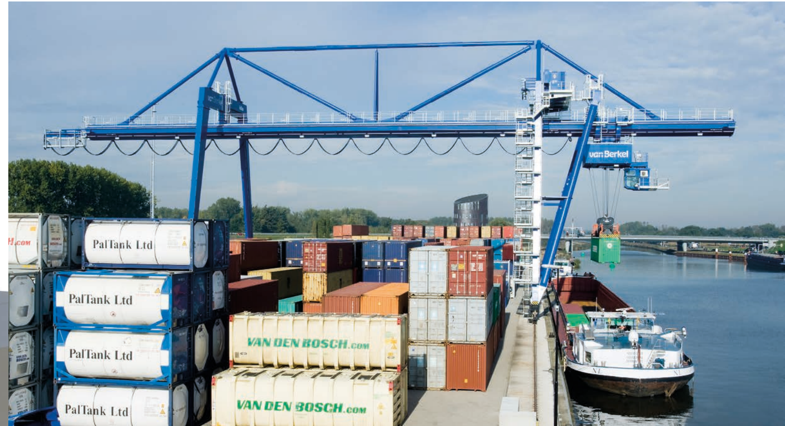
Kuenz Barge Crane with aerodynamic girder at the Van Berkel Logistics Terminal
