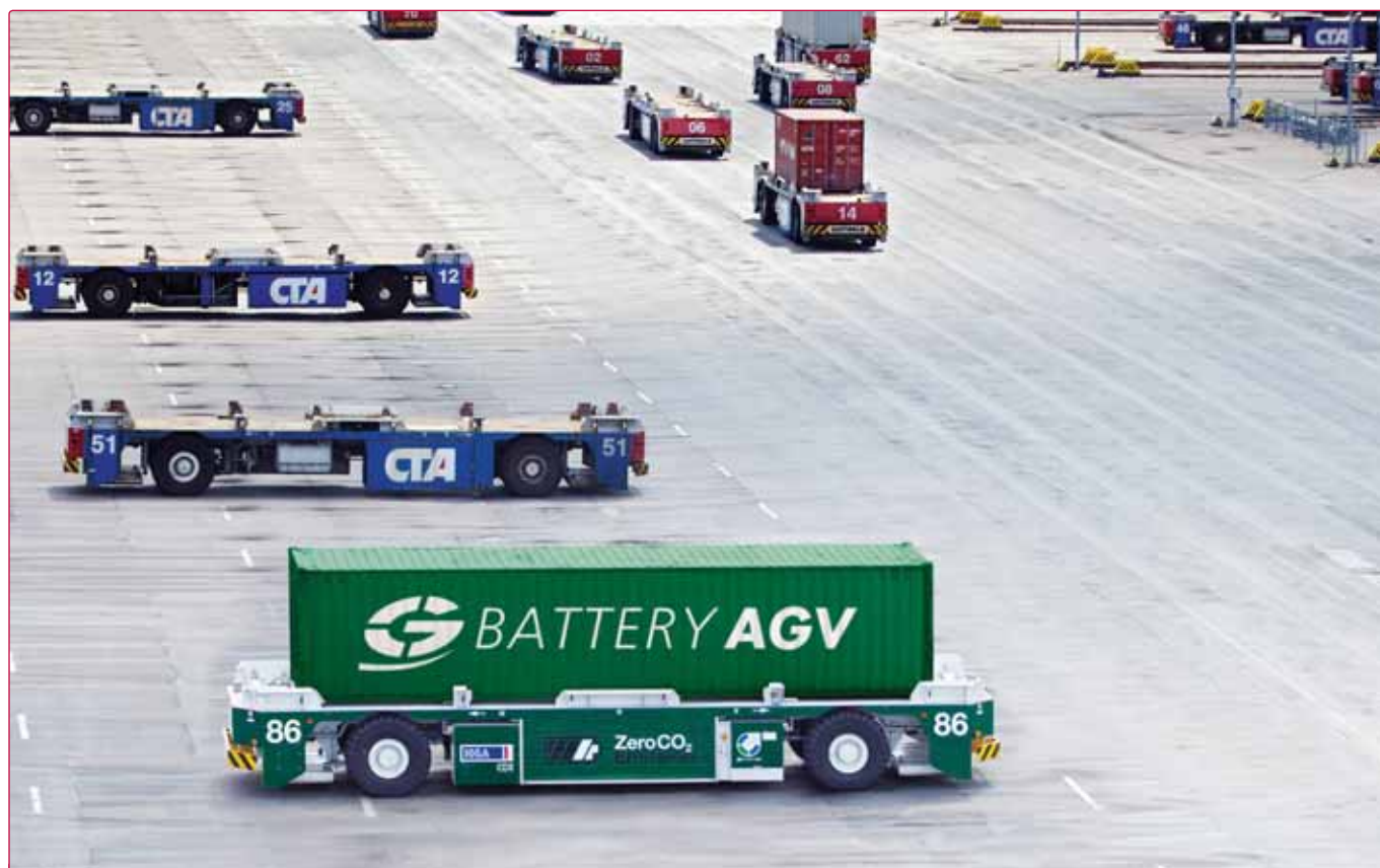
Figure 2. One of two Battery AGV prototypes at the Container-Terminal Altenwerder (CTA), Hamburg.
