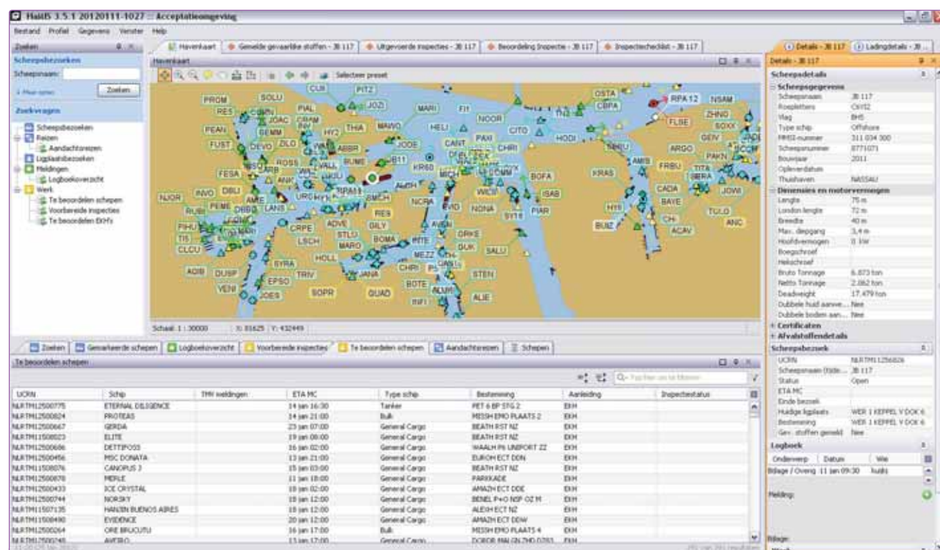
Figure 1. Screenshot of HaMIS (2011). The port and traffic image shows real-time movements of vessels based on radar and AIS data. The supporting data around it provides details on the voyage, the cargo, intended inspections and reference data for each vessel. A mouse click on the vessel in the image immediately makes the vessel, voyage and cargo related data available, it is shown in the tables. Alternatively, a mouse click on a vessel in the table will mark that vessel in the image.
