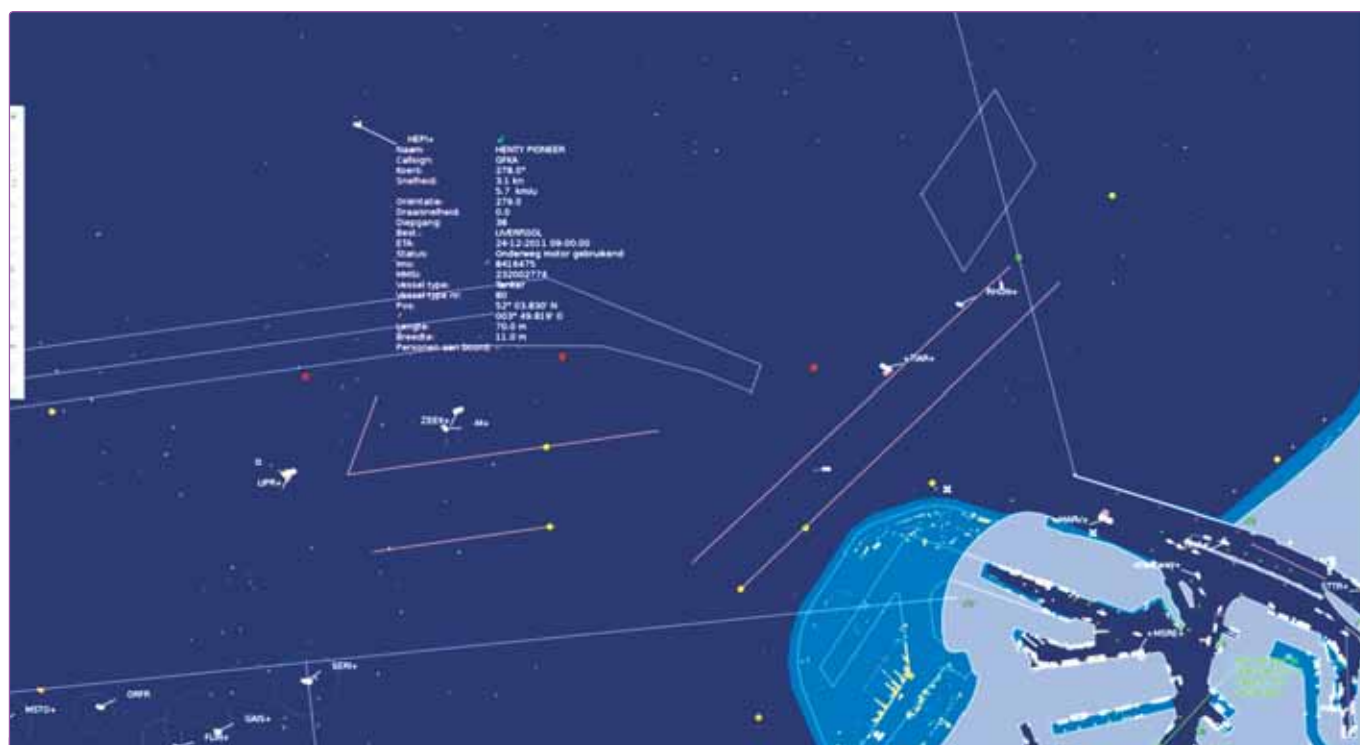
Figure 2. A screenshot of the traffic image based on Aramis (2011). Aramis V3000 is used by VTSO's in the Traffic Centres from January 2012, to monitor the traffic and identify individual vessels, tracks, intended routes, ATA's, ATD's, CPA's and TCPA's, amongst others.
