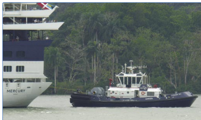
Each tug has at least 60 metric tonnes of bollard pull, an 82 per cent increase over older models.
