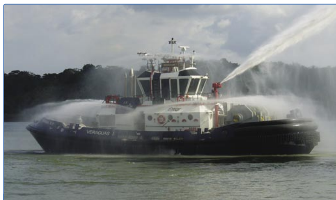
Each tug is equipped with a fire fighting pump, two fire fighting foam tanks and one FFS600 fire fighting monitor.
