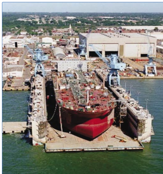
Double-wall tanker in floating dry dock at on-shore facility.
