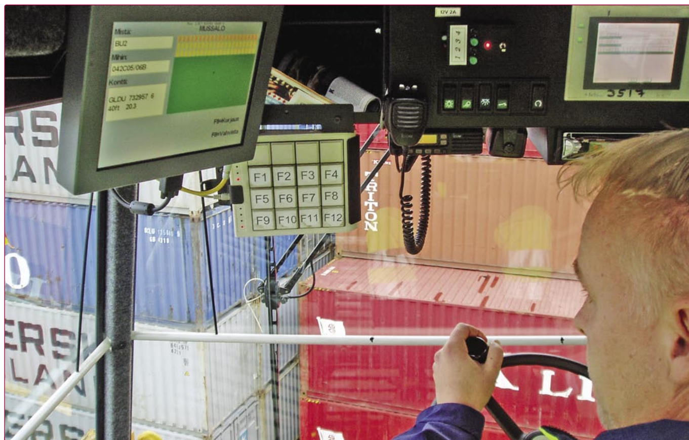
Figure 1. Automatic container position detection system (PDS) not only avoids TOS inventory errors, but also gives the advantage that the driver is not interrupted during the work cycle to operate a keyboard. The straddle driver can thus 'keep the left hand on the steering wheel and the right hand on the spreader controls.'
