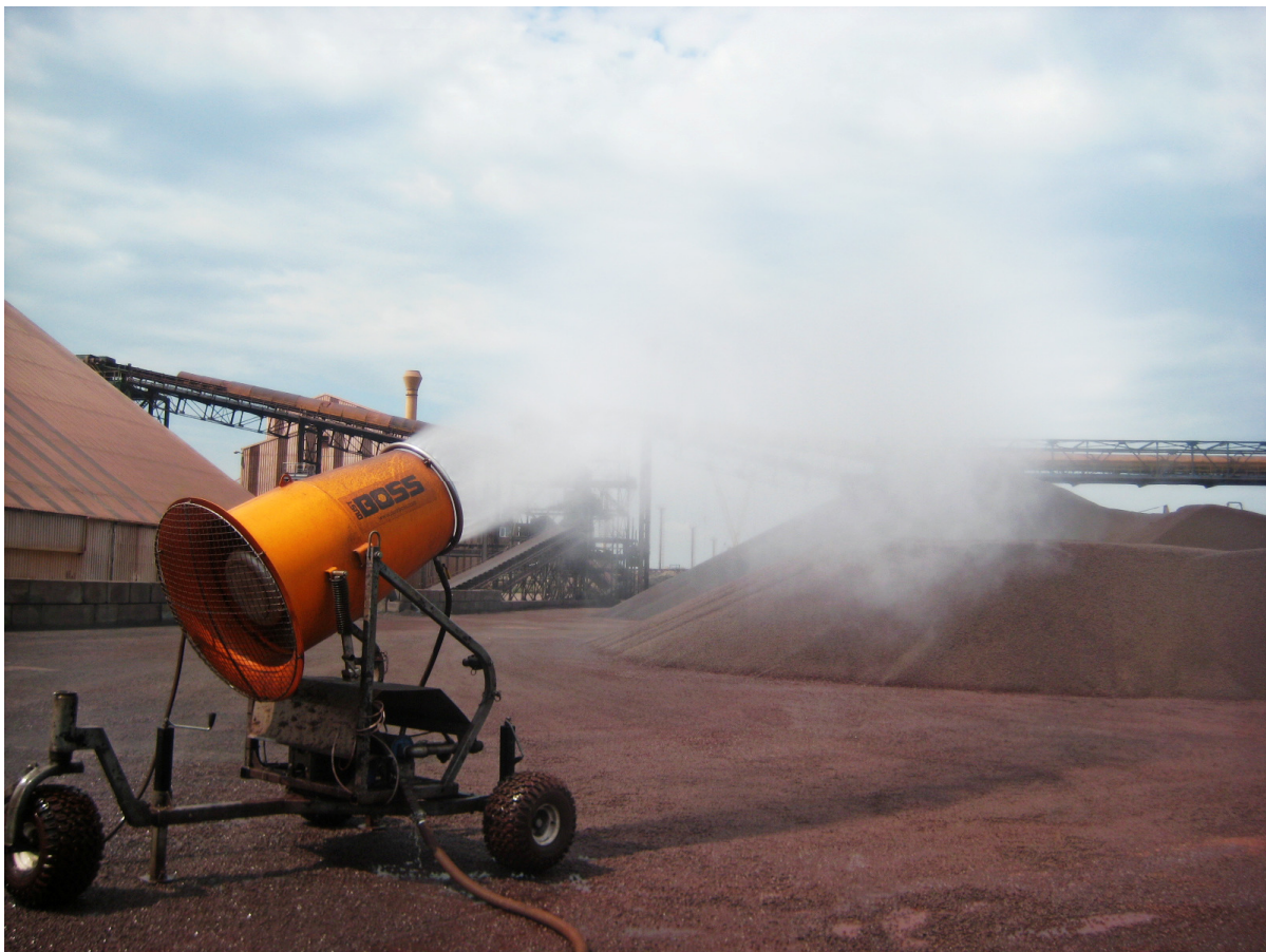
The DustBoss® helps TIS trap airborne particles and prevent dust migration from bulk materials handling operations, including coal, fertilizers and grain. The powerful unit creates a virtual dust blanket over nearly half a football field from a single location, and can be easily relocated on its wheeled carriage.
