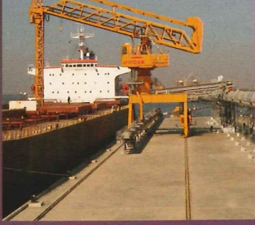
This 1,000tph twin belt system mechanical unloader was commissioned a few weeks ago in Port Qasim in Pakistan.
