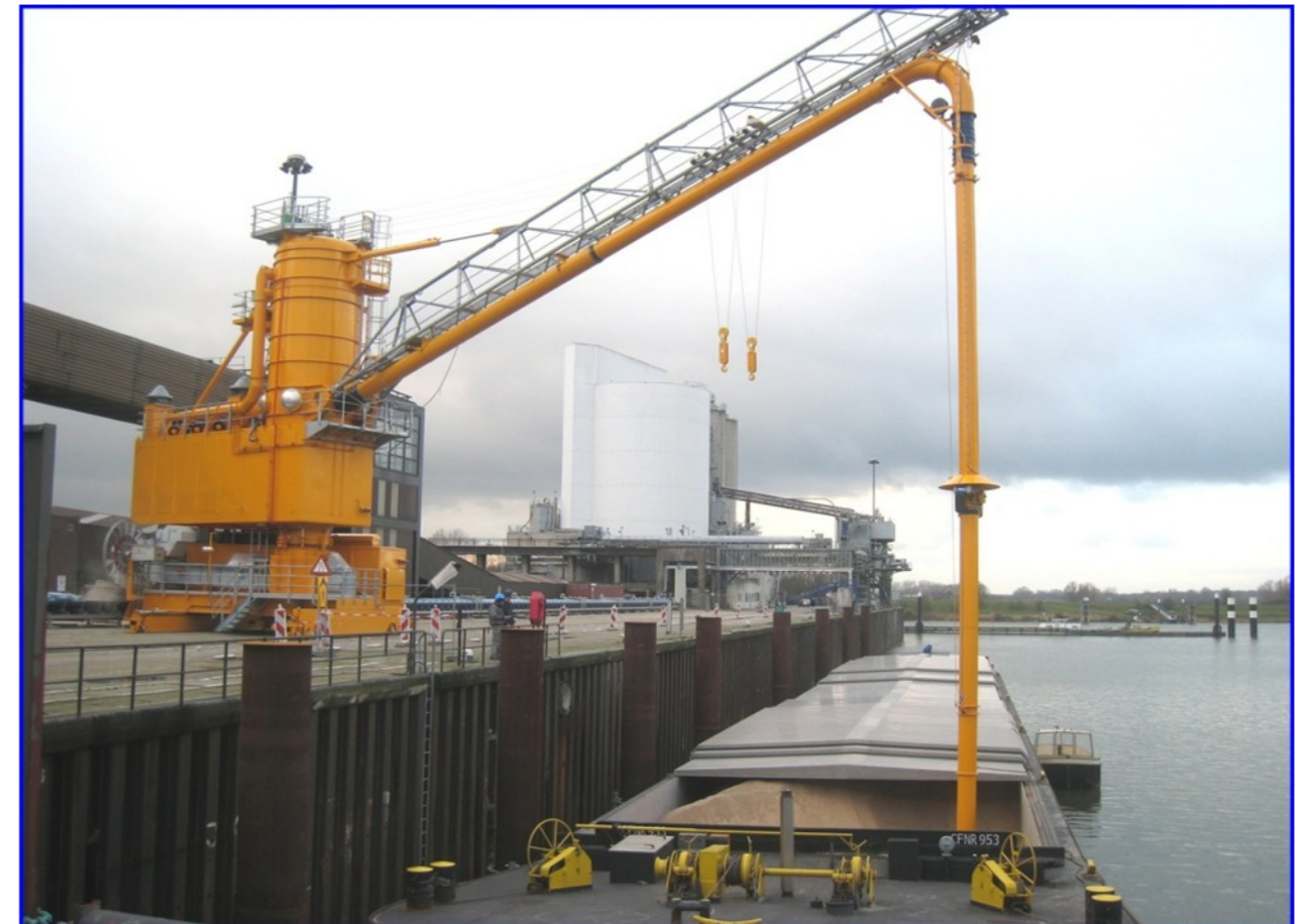
VIGAN barge unloader at ELECTRABEL facilities in Nijmegen – HOLLAND : 500 metric tons per hour.
