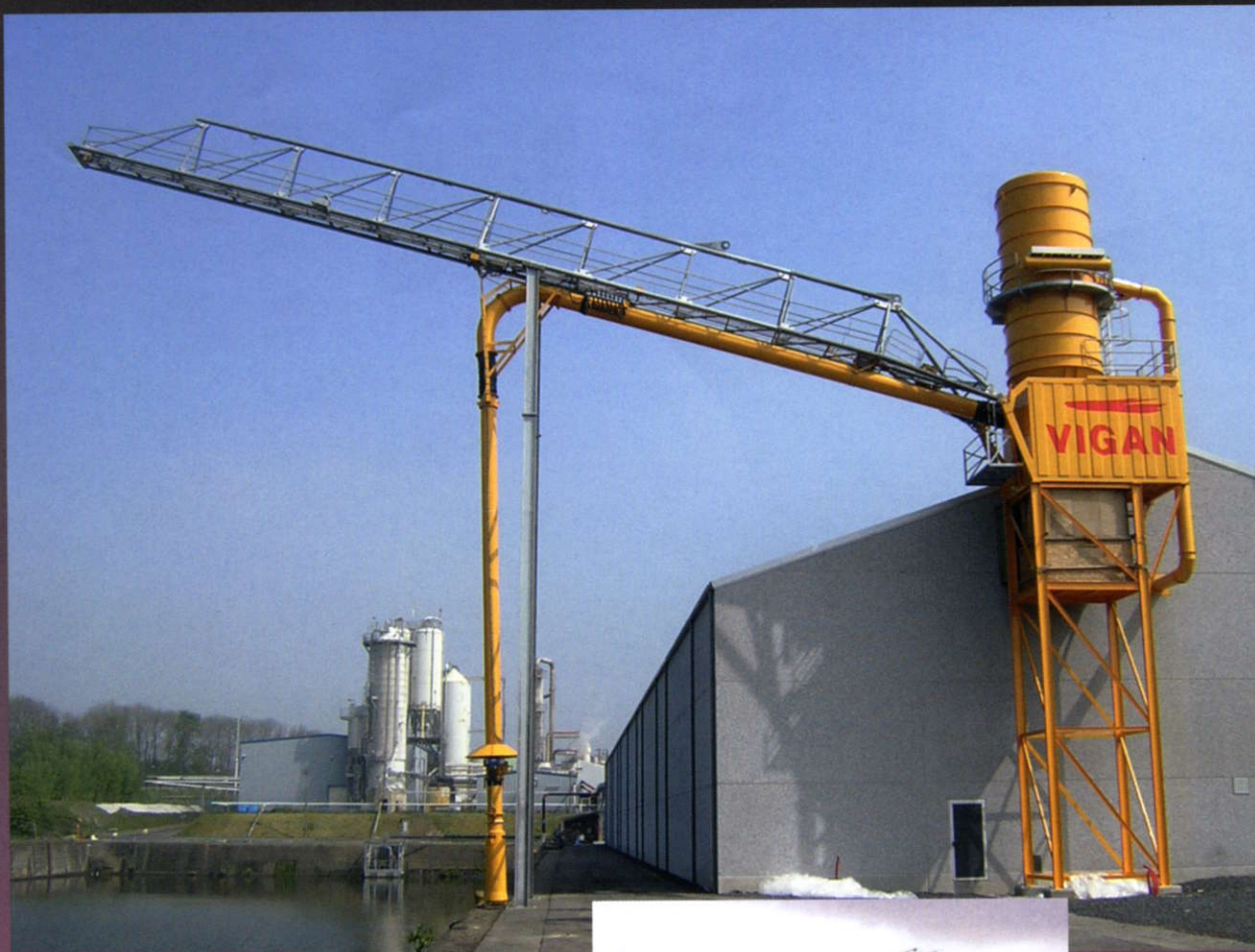
Fixed pneumatic unloaders for barge and handling urea in Belgium: capacity 300tph, delivered in 2009.
