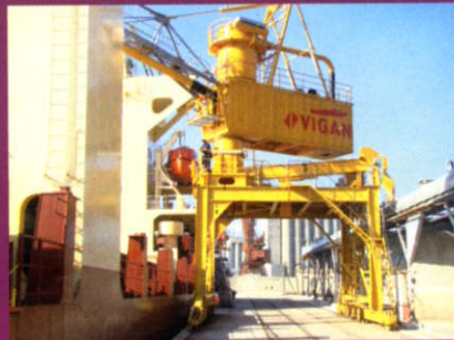
Cuba – port of La Habana: pneumatic unloader on rails with cable reel: capacity 200tph and finally commissioned in 2009. Due to local problems it took about 18 months for erection and final commissioning.
