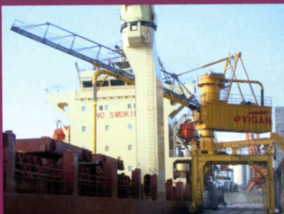
Cuba – port of La Habana: pneumatic unloader on rails with cable reel: capacity 200tph and finally commissioned in 2009. Due to local problems it took about 18 months for erection and final commissioning.
