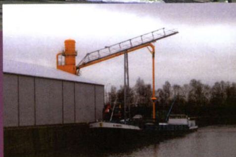
Fixed pneumatic unloaders for barge and handling urea in Belgium: capacity 300tph, delivered in 2009.
